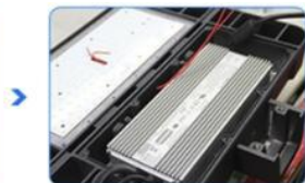
02. Assemble PCB and driver
