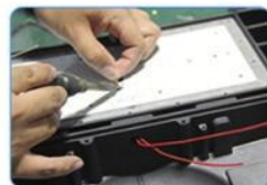
03. Bonding wire/ wire solder
